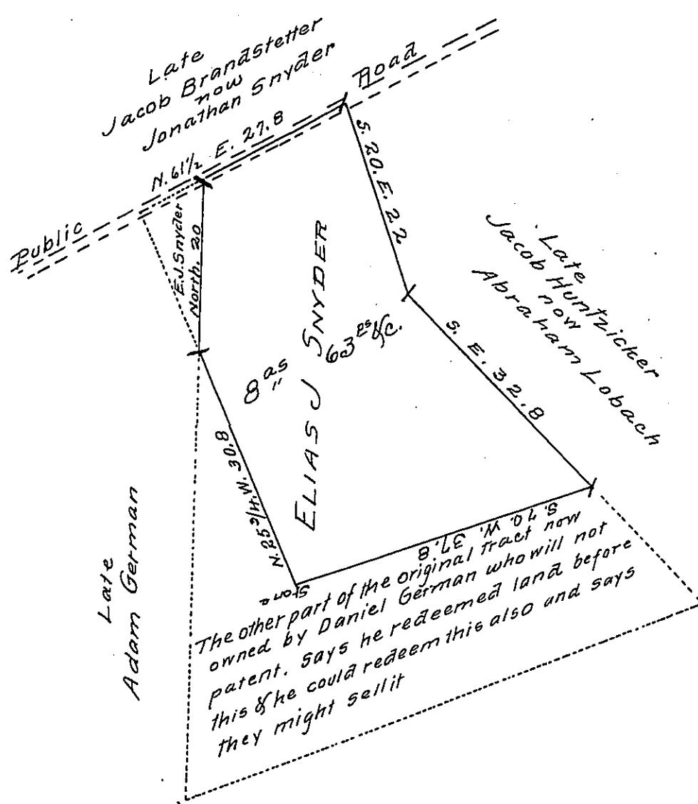
Draft of a tract of land situate in Heidelberg Township Lehigh County containing 8<sup>as</sup> 63<sup>ps</sup> and allowance of six per cent. for roads &c. returned for Elias J Snyder this 19<sup>th</sup> day of Oct. 1874. Being a part of 15<sup>as</sup> 129<sup>ps</sup> of allowance originally surveyed to Adam German by warrant dated April 17<sup>th</sup> 1792
